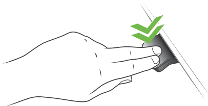
Figure 37: Double-tap to automatically adjust the desk to a favourite position
